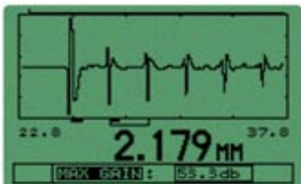
Operator can view thickness and waveform with the optional A-scan mode
