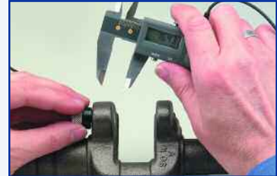
Input Thickness Via Optional Digital Caliper
